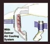
Conventional boots and bandages insulate the horse's tendons and prevent heat escaping. The Dalmar patented cooling system utilizes the high speed cold air hitting the front of the horse's leg to pass through the boot and to cool the tendons while the horse gallops.
